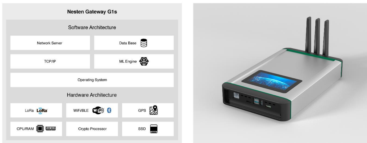
Figure 4 System overview of Nesten wireless node, G1
