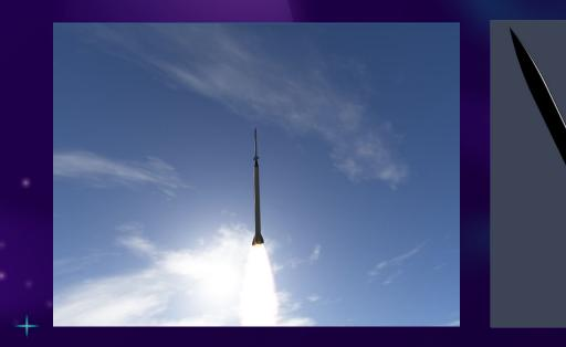
Our test-bed vehicle, capable of up to 45,000 ft of flight is modeled after the sustainer stage of our primary space shot vehicle, the Loki Dart,
