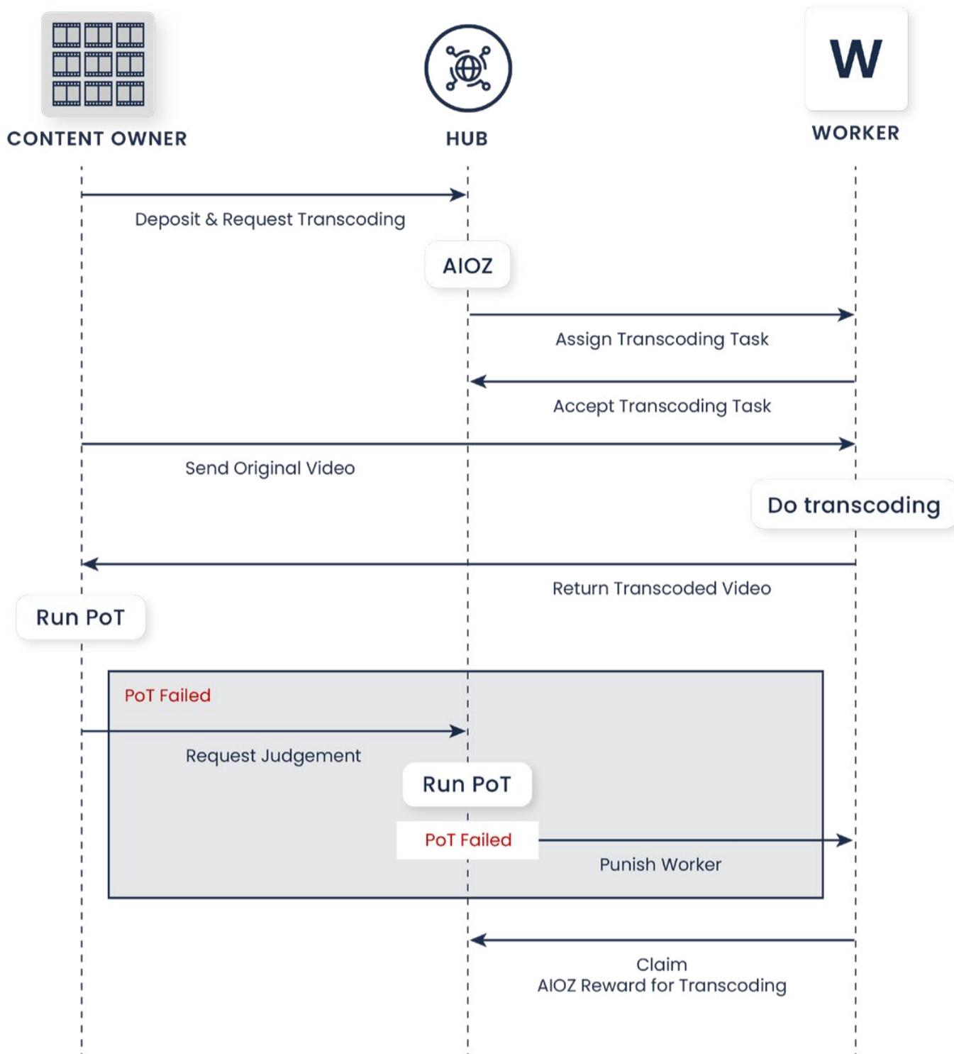
This section will elaborately clarify how Worker Nodes receive the transcoding task and how to prevent them from cheating (Figure). To start with, COs who want to have their videos transcoded will send their request and payment to HUB Nodes of AIOZ CDN. Next, HUB Nodes assess which Worker Nodes can handle COs’ request and assign the task to them. Worker Nodes have the right to accept or to refuse the task assigned by HUB Nodes as well as to freely choose which video segments to handle.
