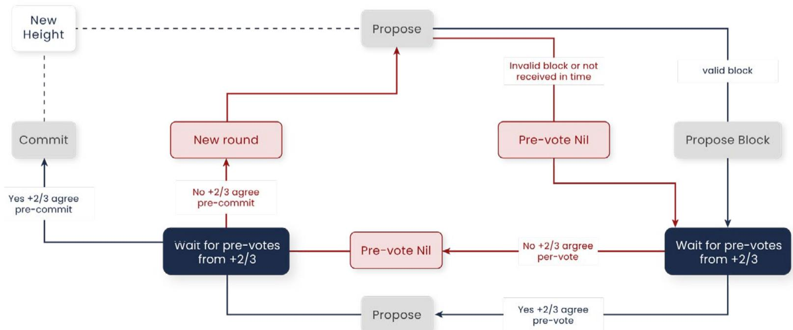
The block proposing process is summarized in Figure : Validators take turns proposing blocks for the transaction and voting on the proposed blocks. The blocks are submitted to the chain with each block on the chain at each height. However, the block may also fail to submit. In this case, the protocol will select the next certifier to propose a new block at the same height and start voting again.
