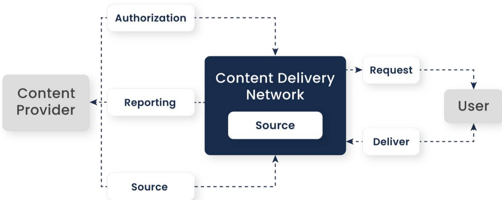
Figure. Model of a typical CDN
