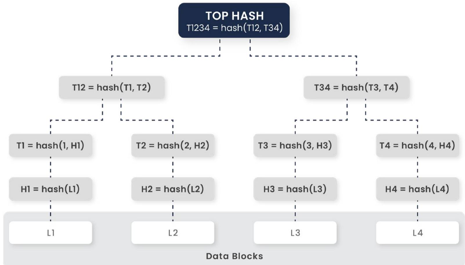
The illustration for a typical Merkle root in AIOZ CDN is shown in Figure. Instead of only 4 blocks shown in Figure, in reality, a video segment contains  $n$  blocks, which  $n$  is computed so that the size of each block ranges from 32 to 64 bits. Via gradual pairing, we will finally achieve a TOP HASH, which is unique for one video segment. In other words, either any changes in any blocks or any block disorders of a video segment will lead to a totally different TOP HASH.
